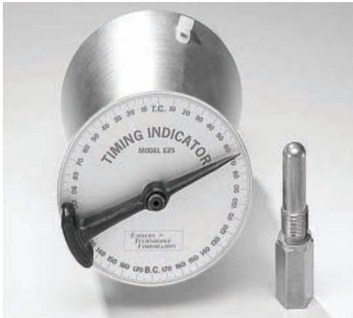
Figure 4—The $360 Pro 3600 digital inclinometer turned out to be off by 3 degrees. The old-fashioned E25 “flowerpot” timing indicator got the job done.
