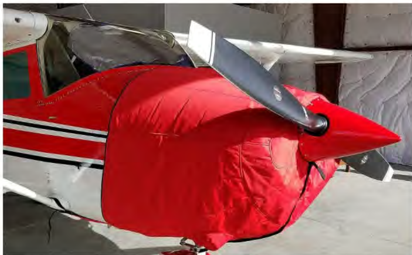
INSULATED ENGINE covers help keep heat from escaping the engine compartment.
