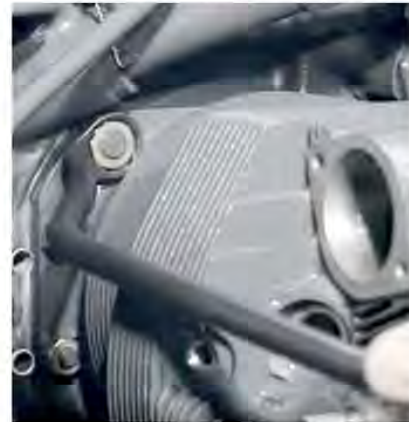
TIGHTENING A CYLINDER hold-down nut is an extraordinarily critical task. Failure to do it exactly right can result in catastrophic engine failure.
