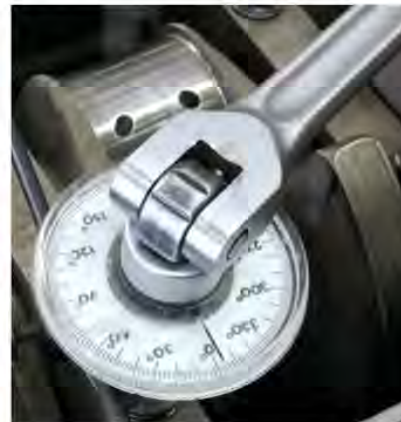
USING THE TORQUE-ANGLE method in an automotive application. Why don’t we do this on our Continentals and Lycomings?
