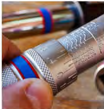
TIGHTENING TO TORQUE is the most common (but inaccurate) way to ensure proper bolt preload.
