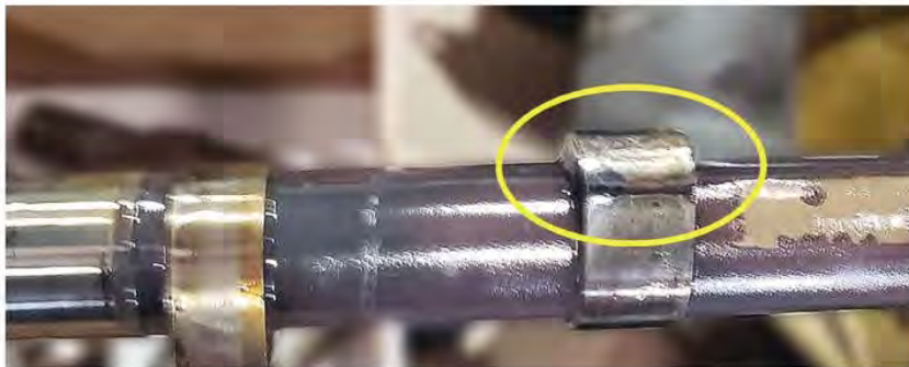
SEVERELY WORN cam lobe.
