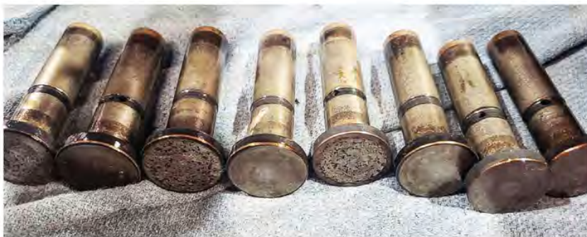
THREE OF the eight tappets are severely spalled.
