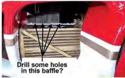
THE T210 OWNER'S IDEAS for modifying his cooling baffles would not have been a good idea.
