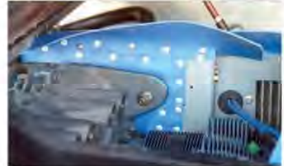
FLEXIBLE SEALS prevent air from escaping through the gaps between the engine-mounted baffles and the cowling, and must curve toward the high-pressure chamber.
