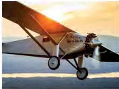
EARLY AIRCRAFT ENGINES were velocity cooled, but this isn't practical for today's high-performance engines and low-drag airframes.
