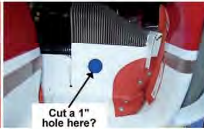
THE T210 OWNER'S IDEAS for modifying his cooling baffles would not have been a good idea.
