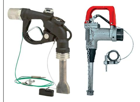
**JET A NOZZLES** have a duckbill design that should not fit into the restricted-size fueling port of a piston aircraft.
