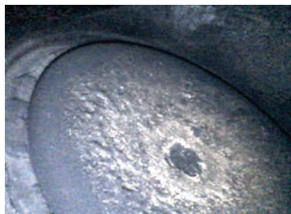
The Lycoming’s exhaust valves all looked fine under the borescope.
