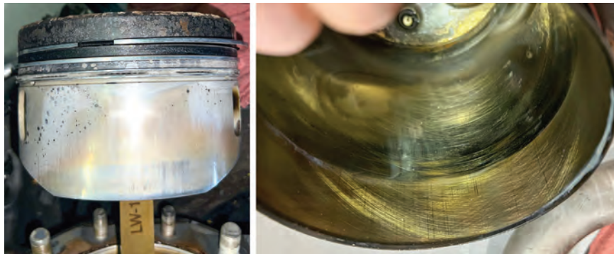
The No. 2 piston was severely clogged with sludge, but the cylinder was in great shape with plenty of visible crosshatch.
