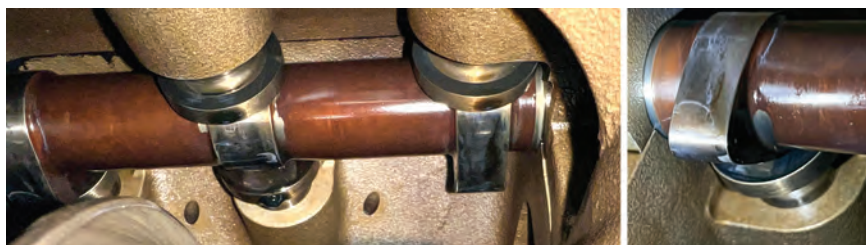
The cam and lifters still looked healthy after 5,000 hours.
