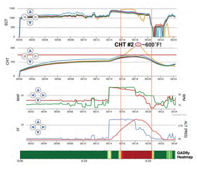
SavvyAnalysis chart of detonation/preignition flight, with GADfly heatmap superimposed.
