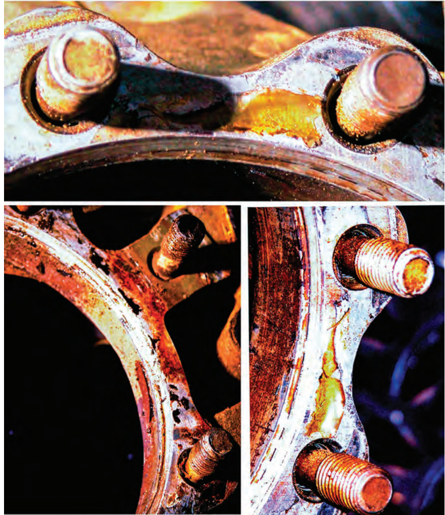
Sealant applied to the cylinder base seals had extruded onto the crankcase mounting decks.
