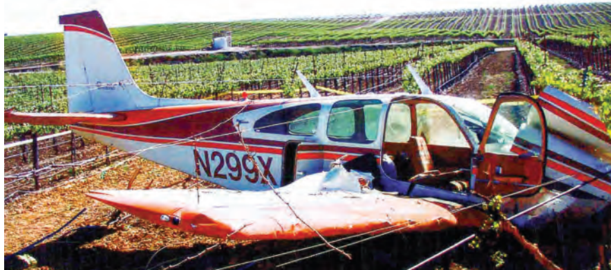
This 1966 Beechcraft Debonair crashed after the #4 cylinder and piston departed the engine in flight.
