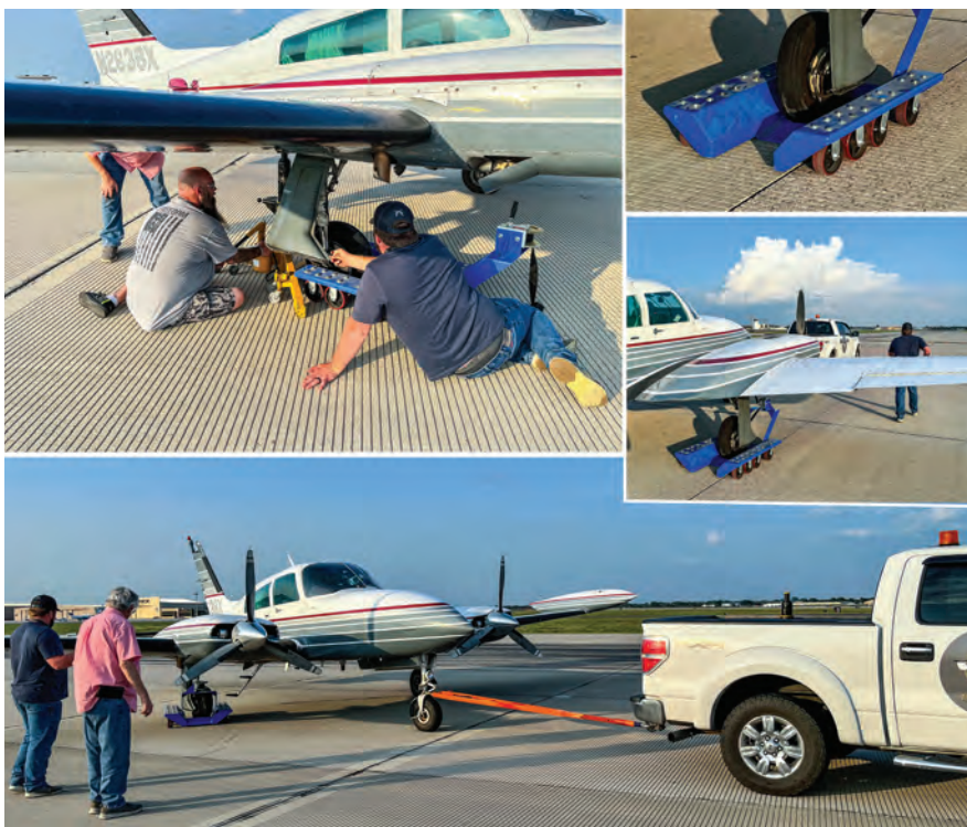
Recovery of '38X featuring Logan, ZZ, yellow jack, blue dolly, orange towbar, and white pickup.
