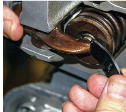
Measuring dry tappet clearance.
