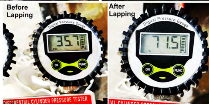
Lapping an exhaust valve in place without removing the cylinder or dropping the exhaust.
