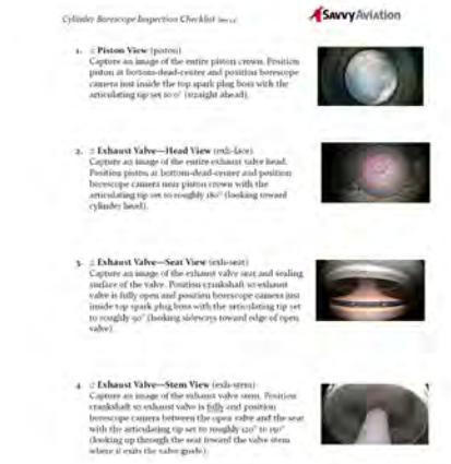
Cylinder borescope inspection illustrated checklist.
