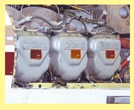
On this big Continental six-banger, mechanics have made note of the compression readings of each cylinder over the years—showing as low as 50/80 pounds at one time. The most recent readings, noted in fresh Sharpie ink, are all in the healthy 70s.
