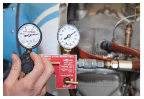
Many aircraft owners and mechanics have placed too much emphasis on compression test readings as a measure of engine airworthiness. The truth is that an engine can have relatively low compression readings while continuing to run smoothly and reliably and make full-rated power all the way to TBO and beyond.
