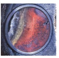
head's large thermal mass and dissipated through its cooling fins (see Figure 2). This "heat sink" arrangement is absolutely essential to the survival of the valve. Without it, the valve face would overheat and selfdestruct quite rapidly.
