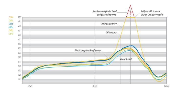
The cylinder head temperature (CHT) data downloaded from the EMax system tells the short tale of the TCM 10-360-ES engine's demise.
