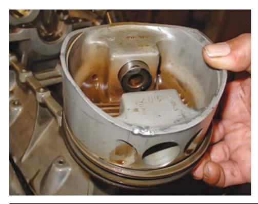
"I wonder how much longer it would have taken for this to cause a catastrophic engine failure? I believe monitoring the engine helped find this, but clearly it would have been found much, much earlier had we been inspecting the pickup screen on a regular basis."
