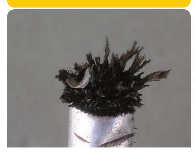
Running a mechanic's magnetic pickup tool around in the drained oil is a good idea for any engine, but particularly for Continental engines where the suction screen cannot be inspected.
