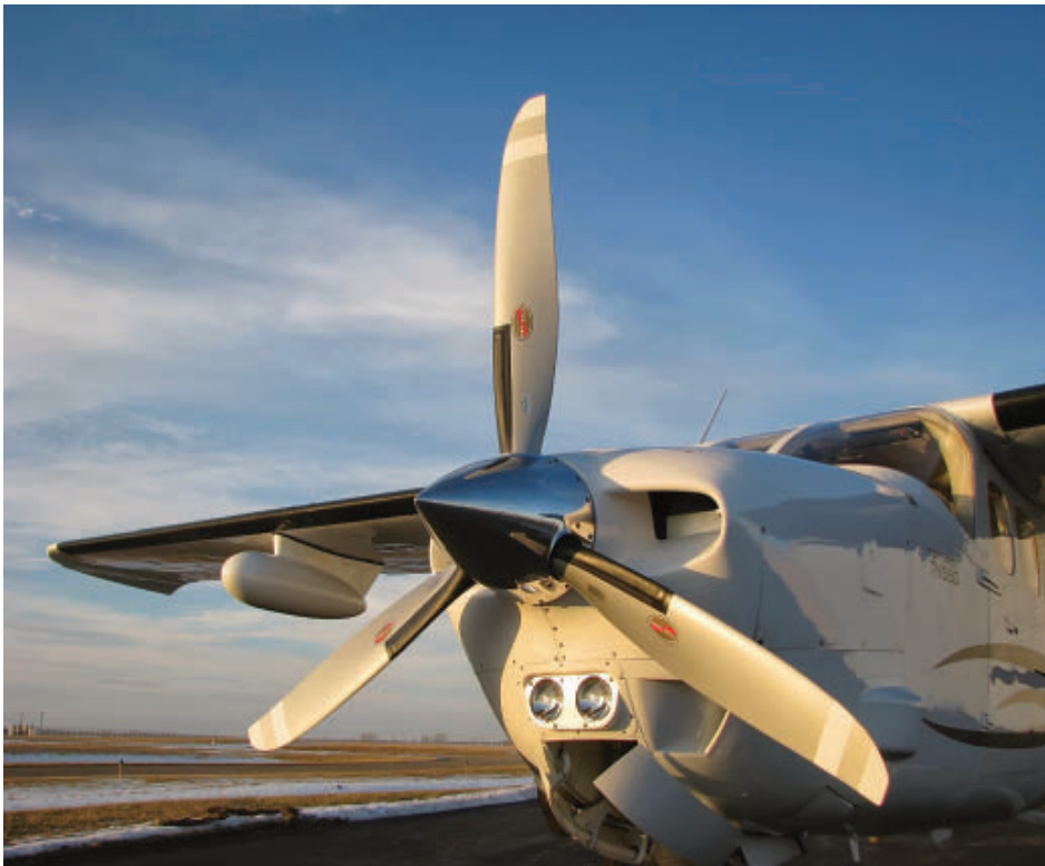
Many mechanics believe that Hartzell propellers are required to be overhauled at TBO because the propeller TCDS references Hartzell's TBO service bulletin. They aren't.
