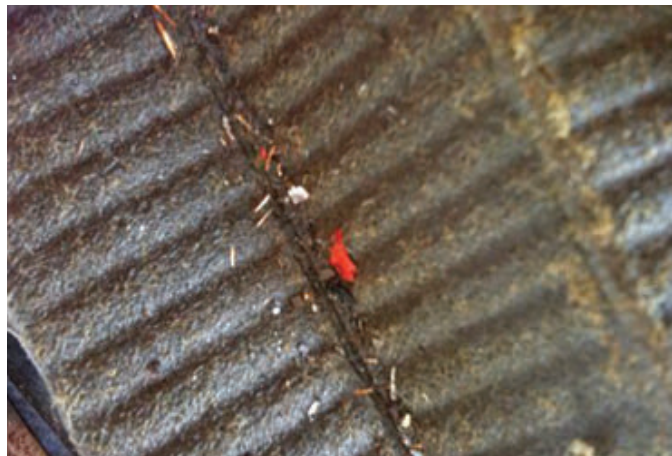
Figure 2. This oil filter media contains hundreds of ferrous metal whiskers, most likely from cam and/or lifter spalling. The engine will likely need a teardown.
