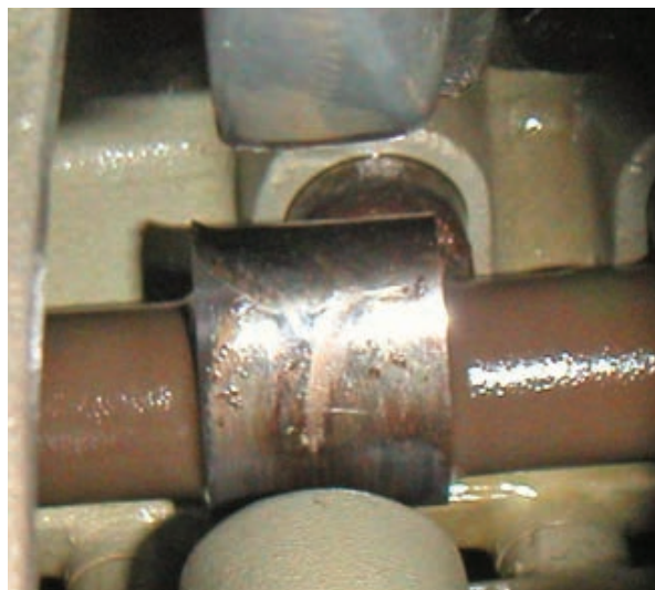
Figure 3. Badly damaged cam lobe found during cylinder removal. It's time!
