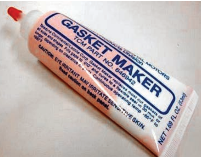
Figure 4—The TCM maintenance manual said that Gasket Maker could be used on "all uncoated oil seals." That turned out to be misleading.
