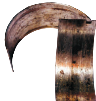
Figure 12—A badly contaminated bearing with large amounts of foreign material embedded in its babbitt overlay.
