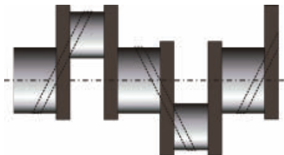
Figure 5—The crankshaft is machined with diagonal oil passages to conduct oil from the main bearings to the crankpin journals in order to lubricate the big-end rod bearings.
