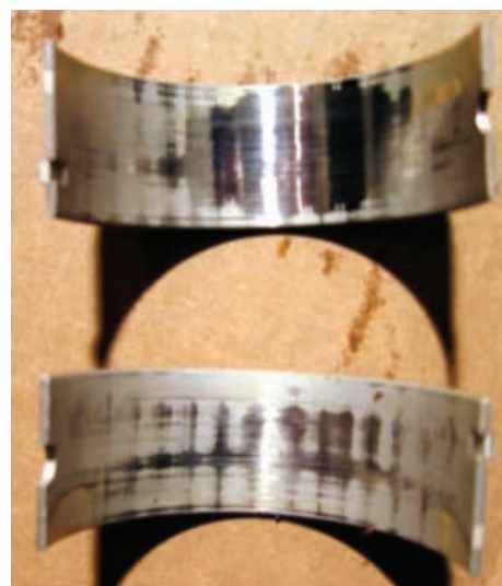
Figure 13—This bearing exhibits severe overload damage, probably due to detonation or preignition.
