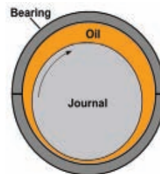
Figure 2—Plain bearings rely on hydrodynamic lubrication to prevent metal-to-metal contact between the rotating journal and the stationary bearing.
