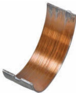
Figure 11—A severely worn bearing with the babbitt overlay almost completely gone.
