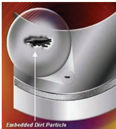
Figure 6—"Embeddability" means the ability of a bearing's running surface to capture particles of dirt, metal, or other foreign materials.
