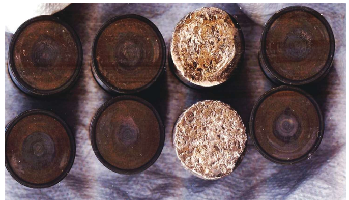
If a Continental-powered aircraft has been inactive for months preceding the pre-buy exam, it may be prudent to pull some lifters and inspect them and the cam lobes for pitting or spalling.
